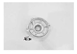
Apply a small quantity of SUZUKI MOLY PASTE to the armature shaft.
