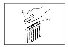
Insert the nozzles of the electrolyte container ⑤ into the electrolyte filler holes of the battery. Hold the electrolyte container firmly so that it does not fall. Do not allow any of the electrolyte to spill.
