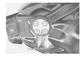
Measure the resistance at each fuel level gauge float position. If the resistance is incorrect, replace the fuel level gauge with a new one.
