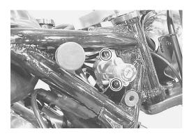
Inspect each switch for continuity with a tester. If any **STARTER BUTTON** abnormality is found, replace the respective switch assemblies with new ones.
