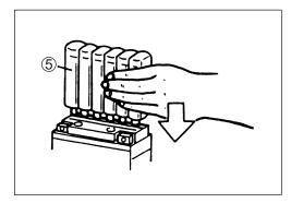
Make sure the air bubbles rise to the top of each electrolyte container and leave the electrolyte container in this position for more than 20 minutes.
