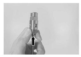
When installing the oil pressure regulator, install the new washer
