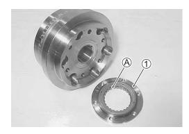
Apply THREAD LOCK SUPER "1303" to the securing bolts and tighten them to the specified torque while holding the rotor with off-set wrench.
