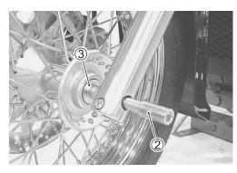
• Remove the brake disc by removing its bolts.
